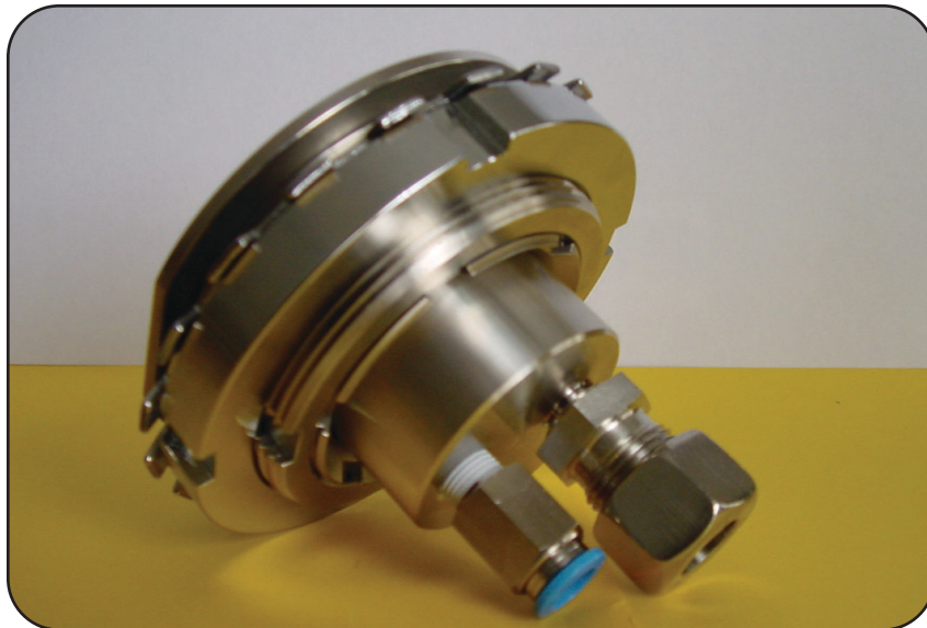
Water and air connections are made at the rear of the PSA Mark3 nozzle. With air assist, the nozzle water spray wetted an area between 0.8 and 4.5 m.
